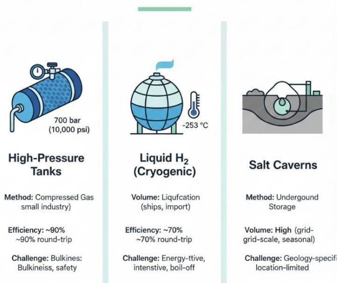
Figure 2 : : Infographic showing hydrogen storage methods: High-pressure tanks vs. Liquid H 2 vs. Salt Caverns
