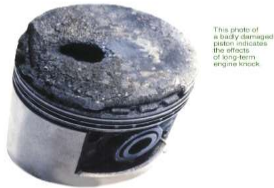
Fig.5. Effect of Knocking In Piston
