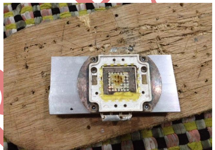
Figure.4. Permanent damage to LED when operated without proper thermal management during the research work
