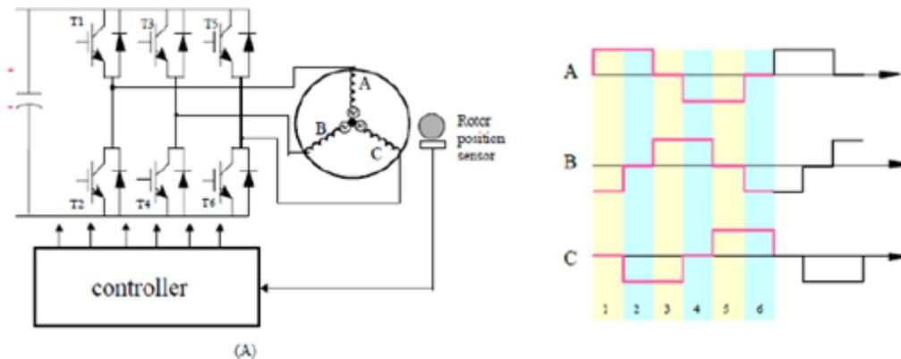
Figure 4. BLDC Motor With Its Drive And Its Three Phase Current Conducting Intervals
