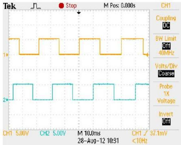
Figure 6. Hall Sensor outputs
