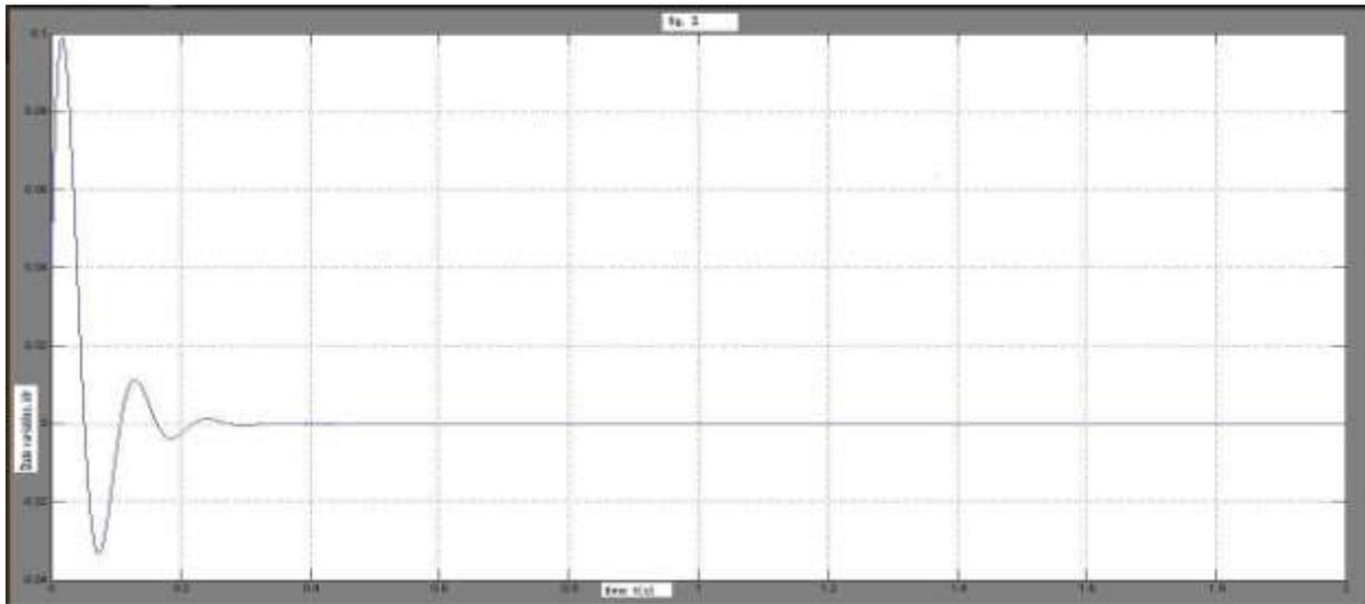
Figure 3 State Variable (idr) with time t(s)
