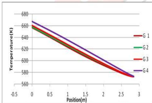
Fig.3 Temperature Plots for all grids of Super heater Section AB
