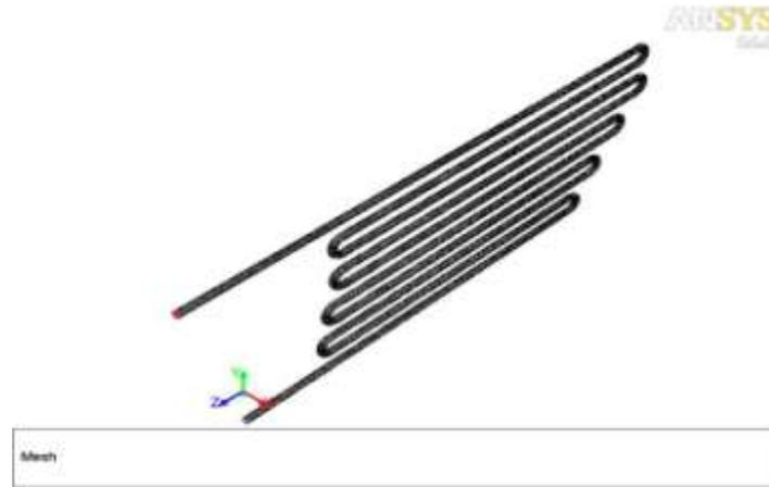
**Fig.2 Meshed Geometry of Super Heater**
