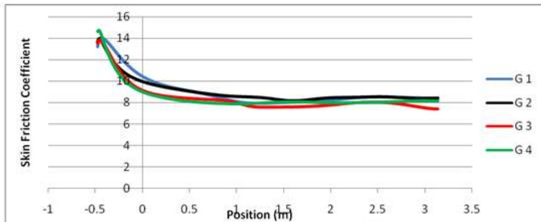
**Fig.9 Skin friction coefficient for all grids of a super heater Section ST**
