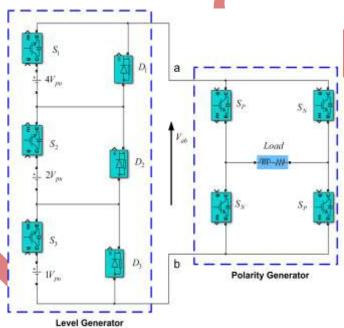
Fig 1: Proposed Asymmetrical 15-Level Inverter Topology
