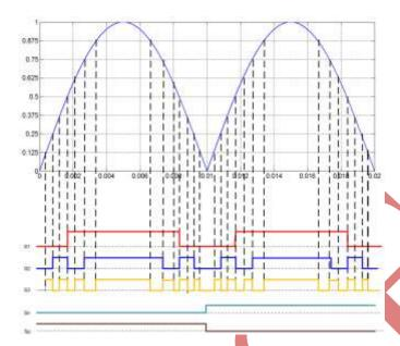
Fig 3: Reference Sine Wave and Gating Signals.
