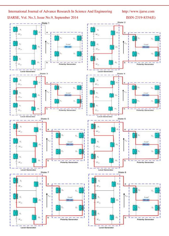
Fig 5: Operating States of the Proposed Inverter.
