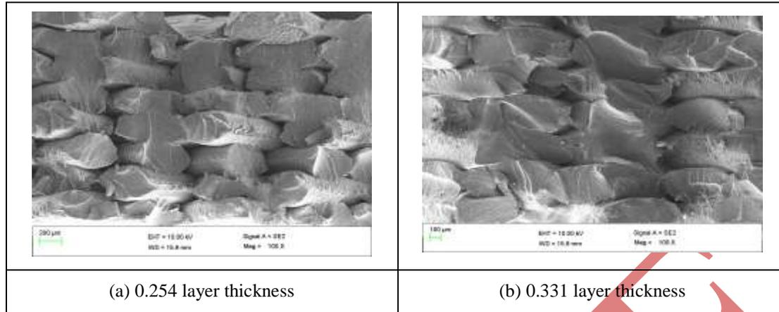
**Figure 5: Fracture Surface of the both layer thickness**
