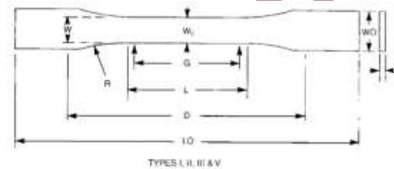
**Figure 1: Tensile specimen according to ASTM D638 .**
