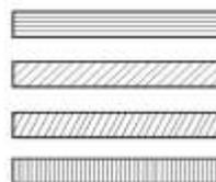
**Figure 2: A schematic shows the variation of raster angle orientation during fabrication.**
