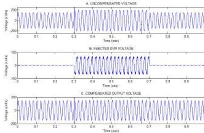
**Figure. 13. Simulation results of Closed Loop Control DVR with 30% swell
