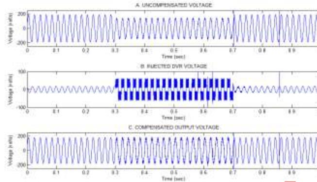
**Figure. 8. Simulation results of Closed Loop Control DVR under 25% sag
