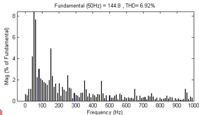
**Figure. 14. FFT Analysis of Closed Loop Control of Voltage Swell Compensation in a DVR System**
