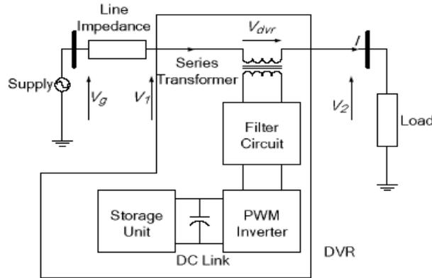
**Figure.1. Block Diagram of General DVR Circuit**
