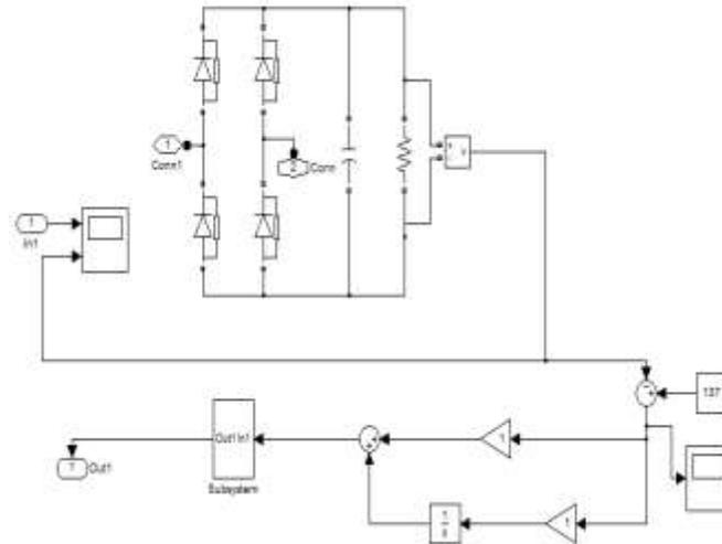
**Figure. 11. Subsystem 1 of Closed Loop Control of Voltage Swell Compensation in a DVR System**
