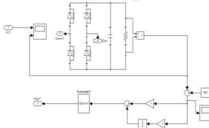
**Figure. 6. Subsystems 1 of Closed Loop Control of Voltage Sag Compensation in a DVR System**
