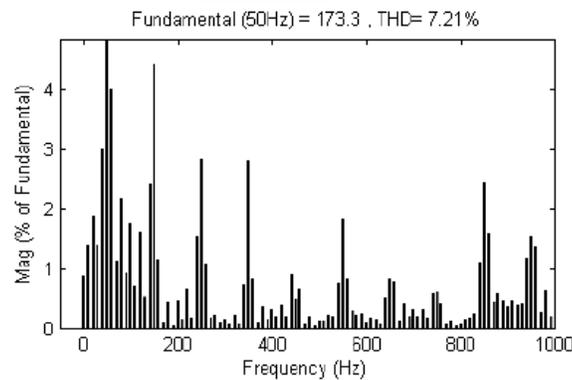
**Figure.9. FFT Analysis of Closed Loop Control of Voltage Sag Compensation in a DVR System**
