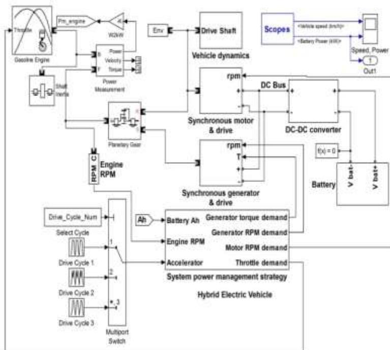
**Fig.-2 Simulation of Hybrid Vehicle**
