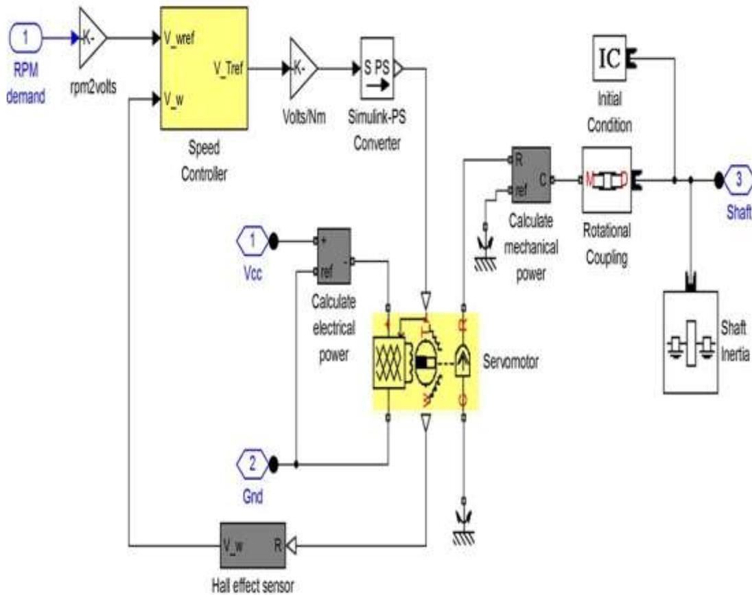
**Fig. 3 Motor and Drive Simulation**
