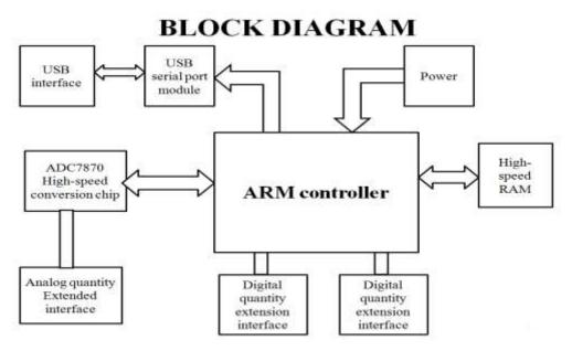
Figure 1: Block Diagram of the Project
