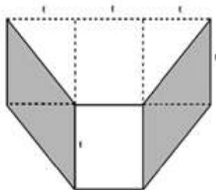
a) Schematic diagram of deformed region in single pressing.
