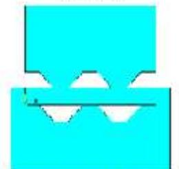
b) Assembly of dies with specimen before pressing
