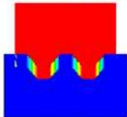
c) Assembly of dies with specimen after pressing
