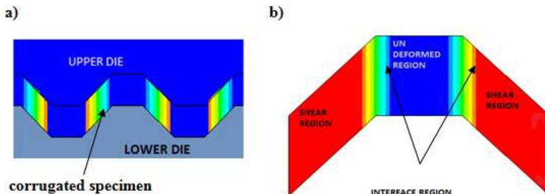
Fig. 6 (A-B) Schematic of Groove Pressing Showing Different Deformation Regions in the Specimen
