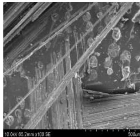
(b) Fiber Failure
