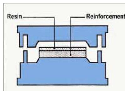
Figure 5: Compression Moulding Machine
