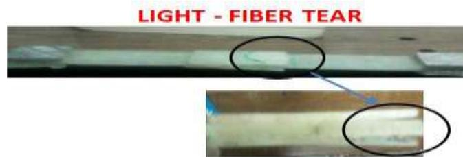
**Figure 14: Light Fiber Tear Failure observed in double lap joints**
