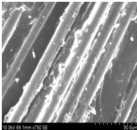
(a) Fiber Tear Failure
