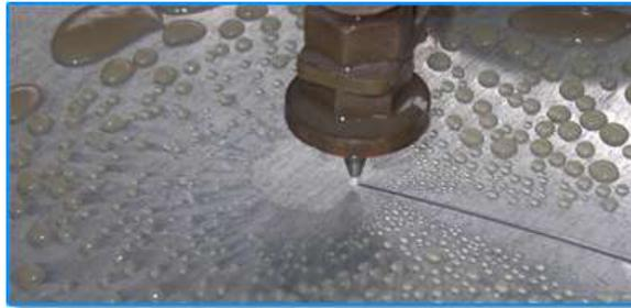
**Figure 6: Water jet cutting**
