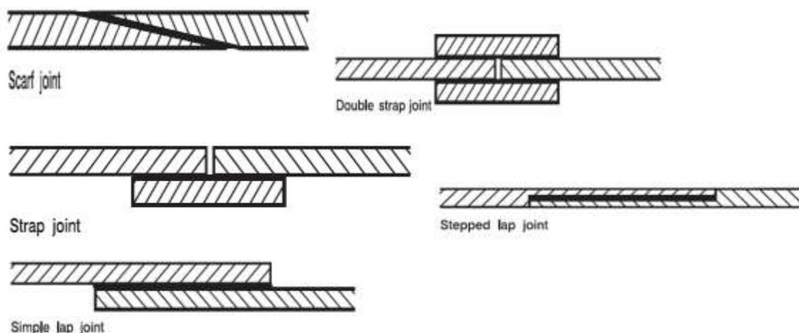
Fig 3: Types of joints.
