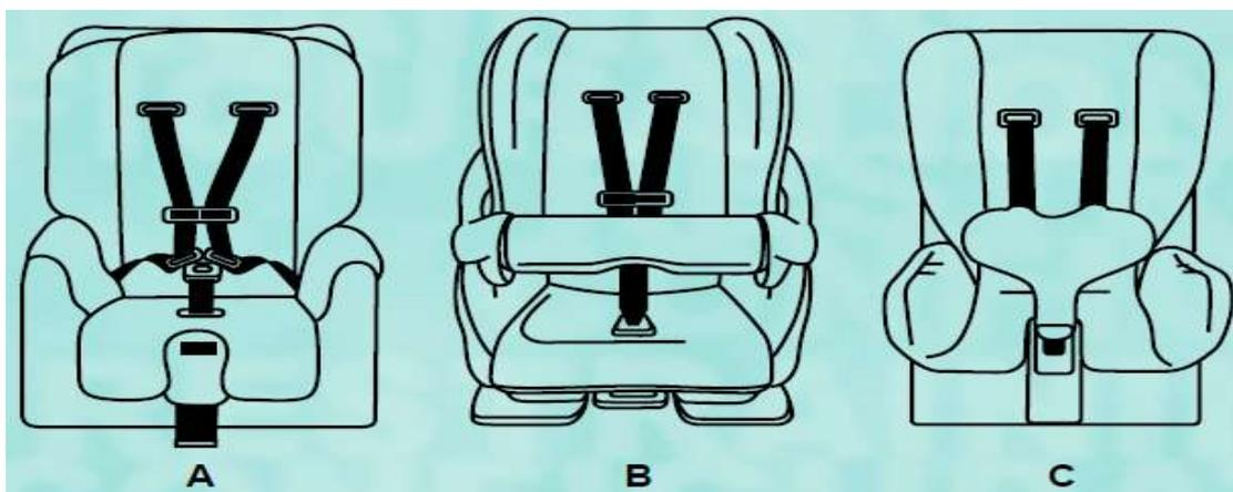
**Fig. 3: Types of harness designations of CRS: (A) 5-point harness, (B) tray shield and (C) T-shield [12]**
