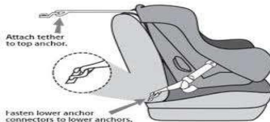
**Fig. 1: Position Of Anchor And Top Tether [12]**
