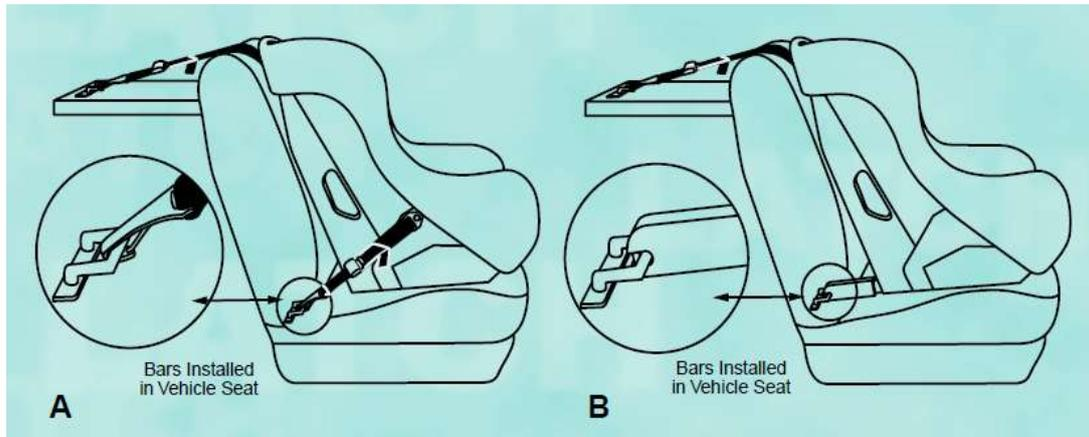
**Fig. 2: (A) Flexible Anchor And (B) Static Anchor [12]**
