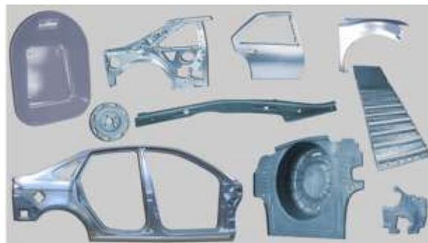
**Figure 5: Example of Stamping Product for Vehicle Manufacturing**
