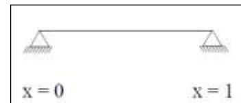
Figure 3.1 simply supported beam
