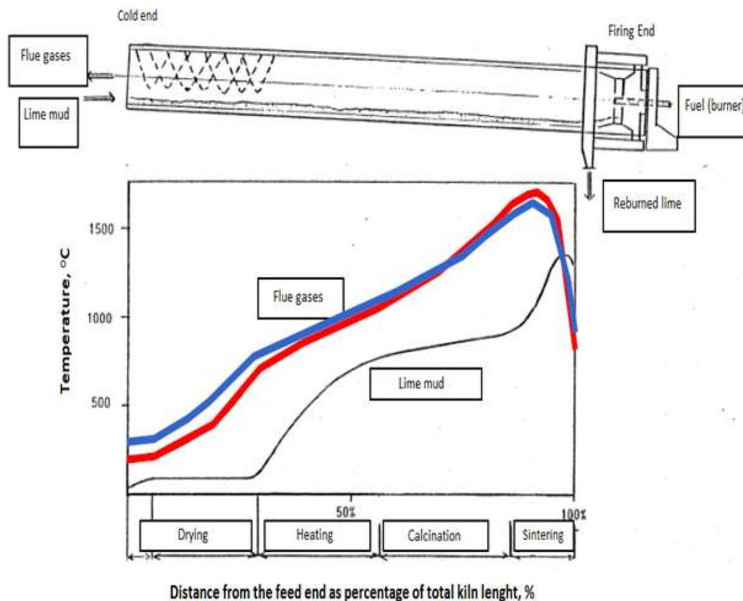
**Figure 4 Lime Kiln Heating Zones**
