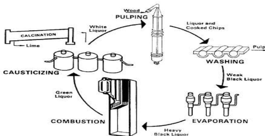
Figure 2 Causticizing process of the pulp mill recovery circuit
