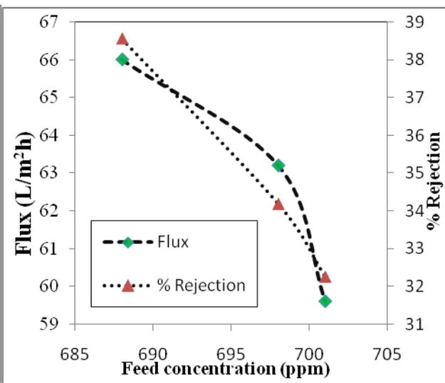
**Fig. 9: Effect of Feed Concentration on Flux and Rejection of NF membrane at 21 kg/cm<sup>2</sup>**
