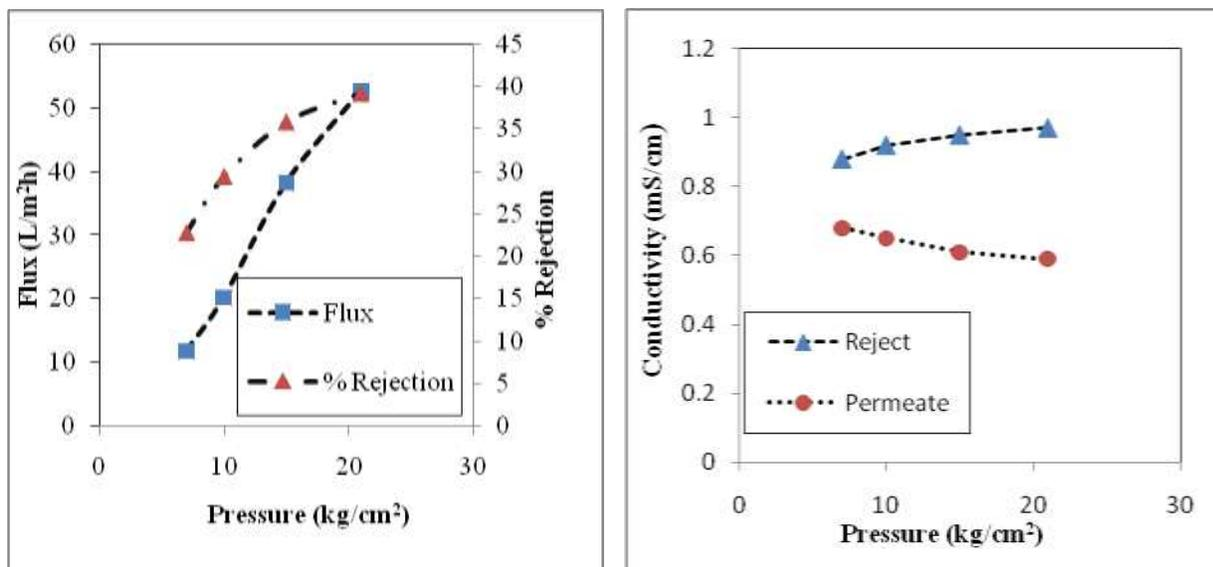
**Fig. 7 a: Effect of Pressure on Flux and % Rejection for Bore well Water**      **Fig. 7 b: Effect of Pressure on Permeate and Reject Conductivities**
