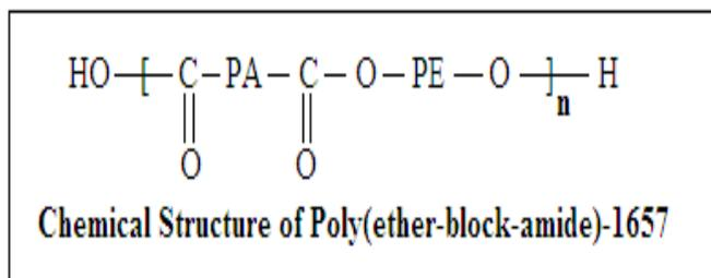
Fig. 1: Chemical Structure of PEBAX-1657
