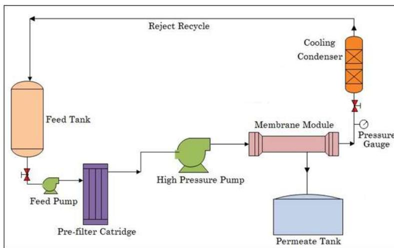
**Fig. 2: Process Flow Diagram of NF system**
