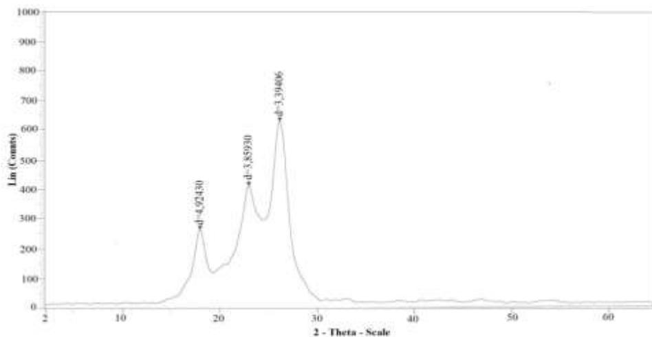
**Fig. 4: XRD Spectra of NF membrane**
