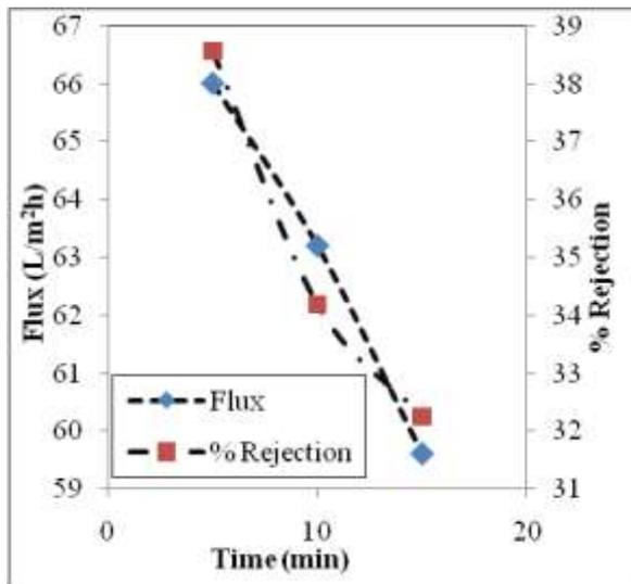
**Fig. 8: Effect of operating time on NF Membrane on Flux and % Rejection for bore water**
