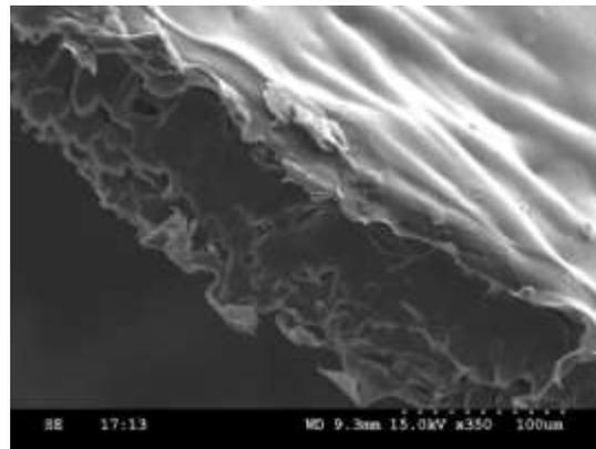
**Fig. 6 a: SEM Image of NF Membrane Surface**
