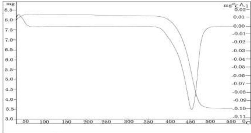
**Fig. 5: TGA Curves of NF membrane**
