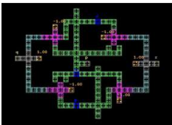
Fig 7 Proposed layout of Fredkin gate
