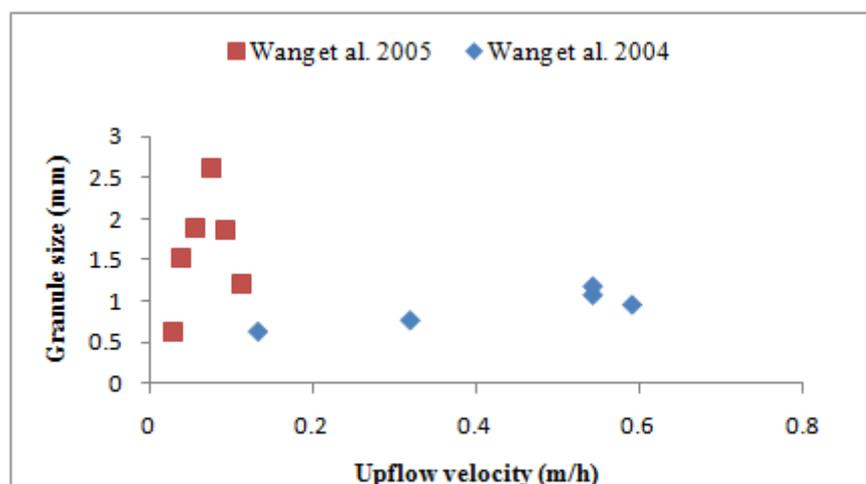
**Fig.2 Variation of upflow velocity ( $V_{up}$ ) with granule size**
