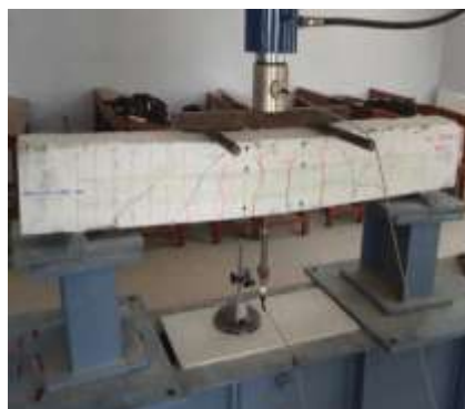
Fig. 8: Specimen under Loading
