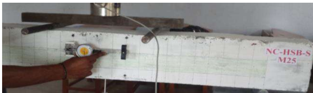
Fig.14: Strain Measurement under Loading
