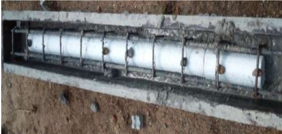
Fig. 4: Beam with Circular Expanded Polystyrene Foam in Tension Zone
