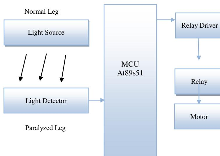
Fig. 1: Block diagram of light sensing mobile shoe
