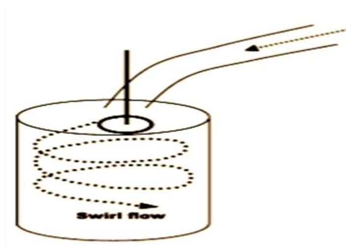
**Fig.1: swirling motion in an engine cylinder**
