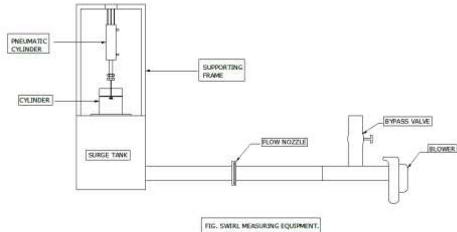
**Fig.2: Block diagram of swirl measuring equipment experimental set up**
