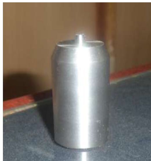
Fig 3 a) Tool pin profile
