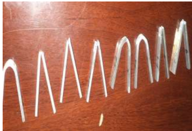
Fig 6 a) Typical bended specimens of Face bend
