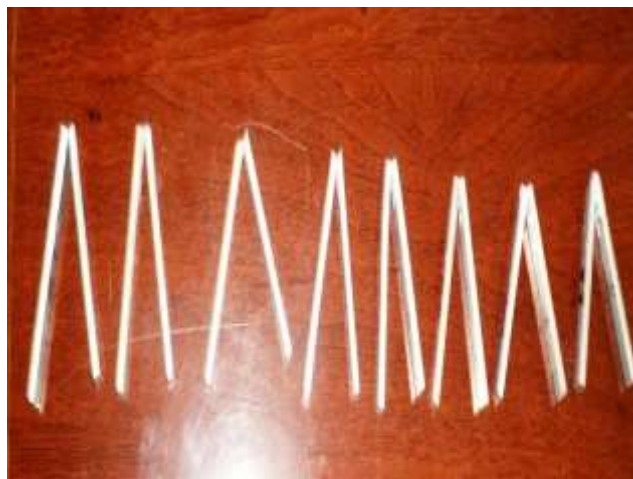
Fig 6 b) Typical bended specimens of Root bend
