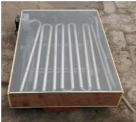
Figure 1. Solar Air Collector For Space Heating
