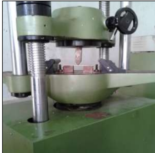
Figure3 : Initial Geometry Of Punch, Die And Sheet.
