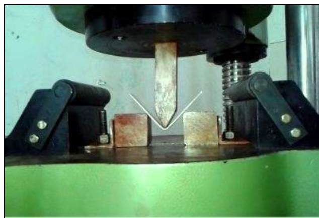
Figure: 4 Deformed Sheet at 100% Displacement
