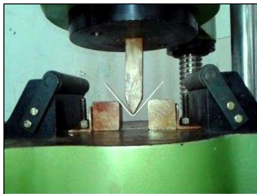
Figure3 : Initial Geometry Of Punch, Die And Sheet.
