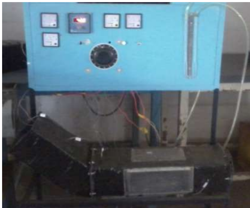
Fig. 2.2 Experimental Setup (Inlet at 45^{\circ} Inclination)
