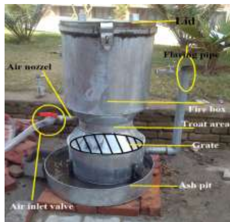
Fig: Construction and Parts of Gasifier
