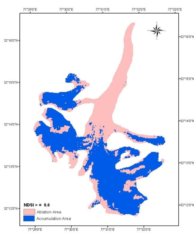
**Fig4.b. Separation of Accumulation and Ablation area of glacier by applying threshold of 0.6 on NDSI map of 25 Aug 2005**
