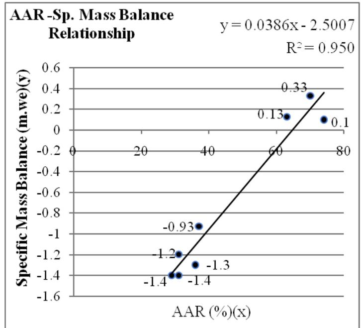
Fig3 Mathematical Model Derived from the Relationship Between Mass Balance and AAR with  $y=0.0386*x - 2.5007$  with Coefficient of Correlation is 0.95.
