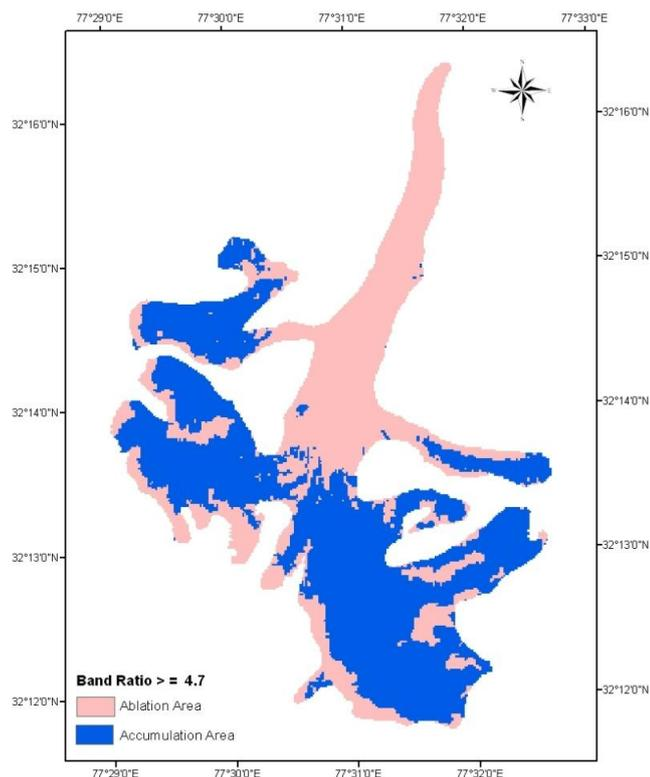
**Fig4.a. Separation of Accumulation and Ablation area of glacier by applying threshold of 4.7 on Band ratio map of 25 Aug 2005**
