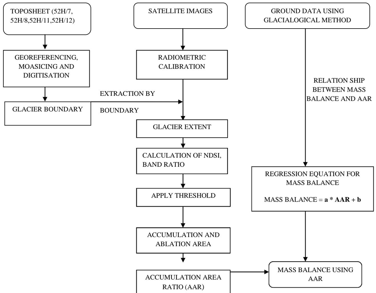
Fig. 2: Overall Methodology for Estimating the Mass Balance Using AAR Method
