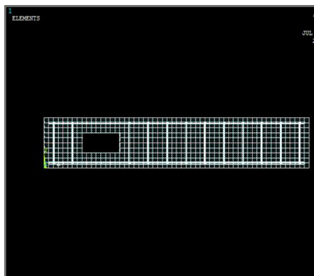
Fig. 11: Model Of Shear Zone Opening
