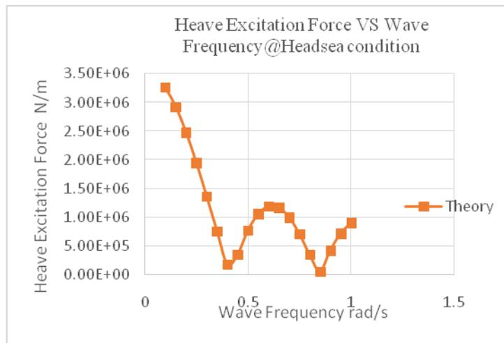
**Figure 1: Heave Excitation Force Semisubmersible Hull**
