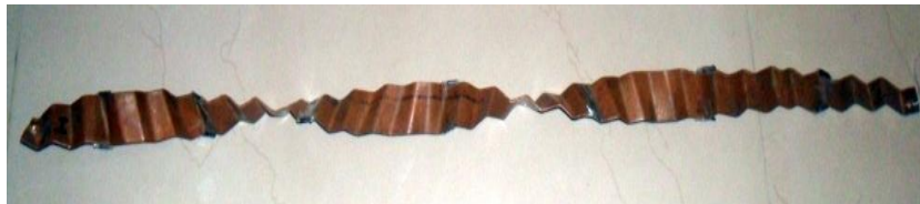
Fig 6.(a) : Copper wavy insert TR-8.83, WW-16 mm
