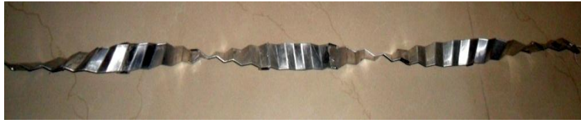
Fig 5 (b): Aluminum wavy insert TR-9.79, WW-13 mm
