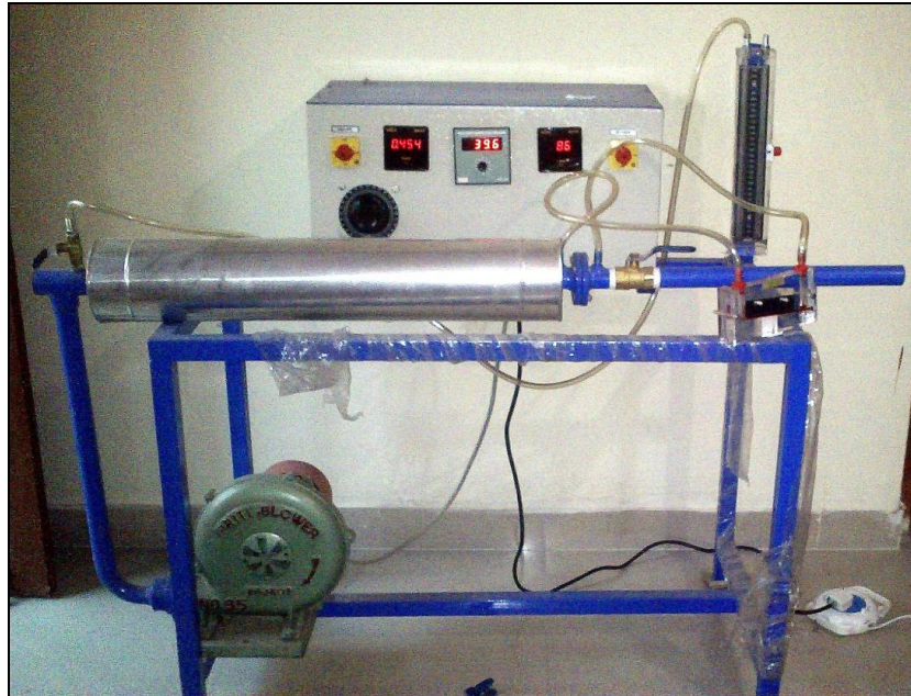
Fig 1: Experimental Set up for Forced Convection
