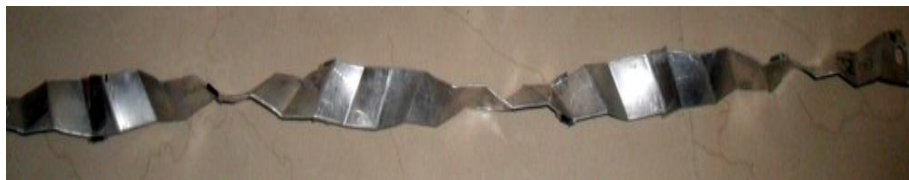
Fig 4 (c): Aluminum wavy insert TR-9.375, WW-24 mm
