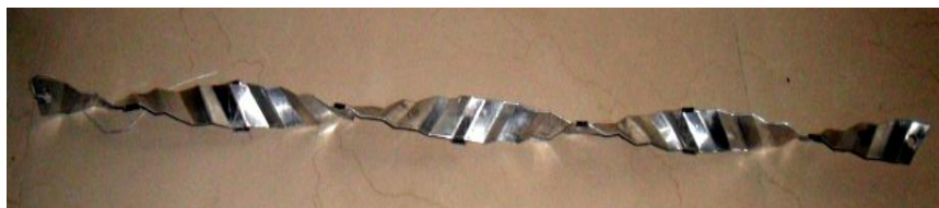
Fig 5 (a): Aluminum wavy insert TR-8.33, WW-13 mm
