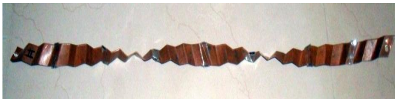
Fig 6.(b) : Copper wavy insert TR-9.79, WW-16 mm
