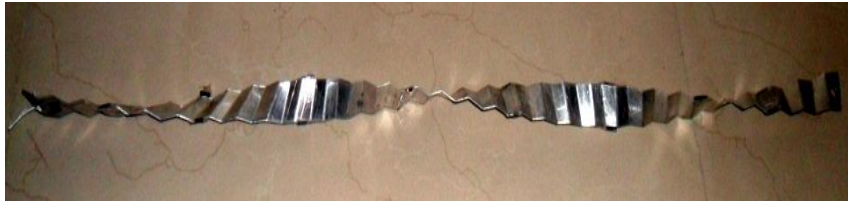
Fig 5 (c) : Aluminum wavy insert TR-10.42, WW-13 mm
