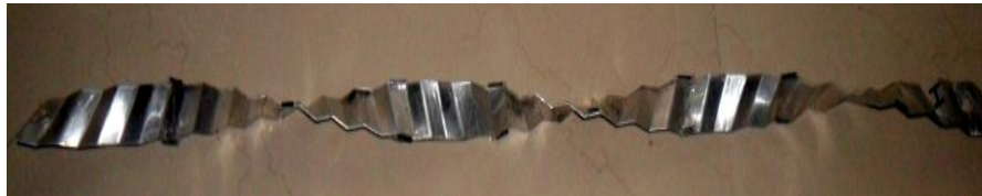
Fig 4 (a) : Aluminium wavy insert TR-9.375, WW-13 mm
