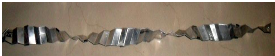
Fig 4(b) : Aluminium wavy insert TR-9.375, WW-16 mm
