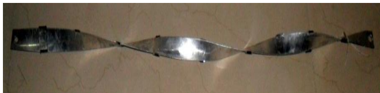
Fig 7 : Aluminum plane twisted tape insert TR-9.375
