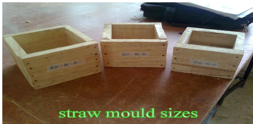
Figure 2.1: Wooden Mould of Straw Bale.
