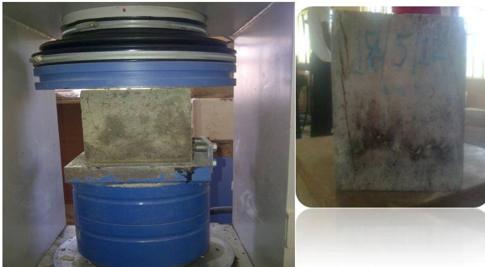
Figure 2.6: Plastered Straw Bale Under Compression and its Mode of Failures.
