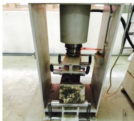
Fig.7- Flextural Strength Teasting
