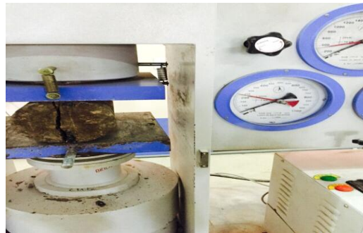
Fig.6- Split Tensile Strength Testing
