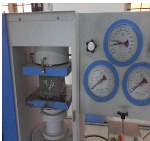
Figure.5 Compression Testing of Geopolymer Concrete Cube
