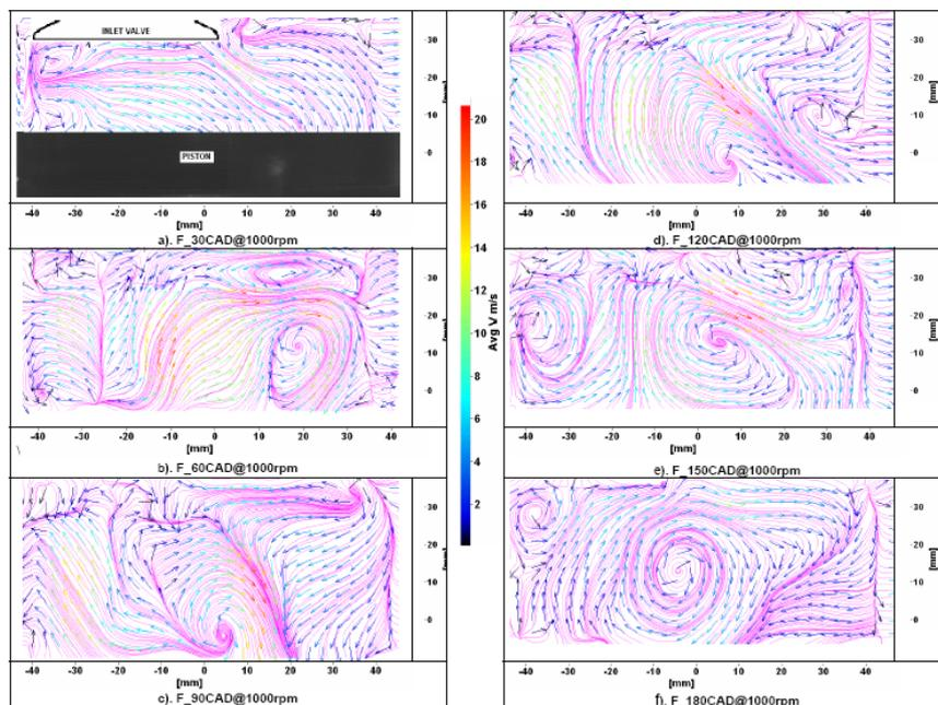
**Fig.3 The Ensemble Average Velocity Vector Fields of Flat Piston During Intake Stroke**
