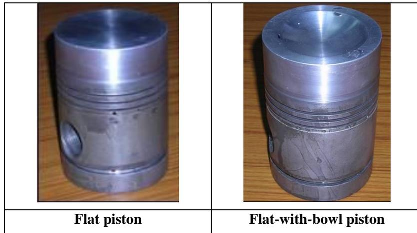
**Fig.2 Flat and Flat-with-Bowl Pistons**
