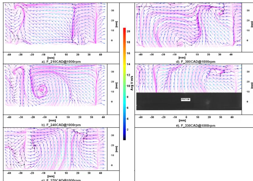
Fig.5 The Ensemble Average Velocity Fields of Flat Piston During Compression
