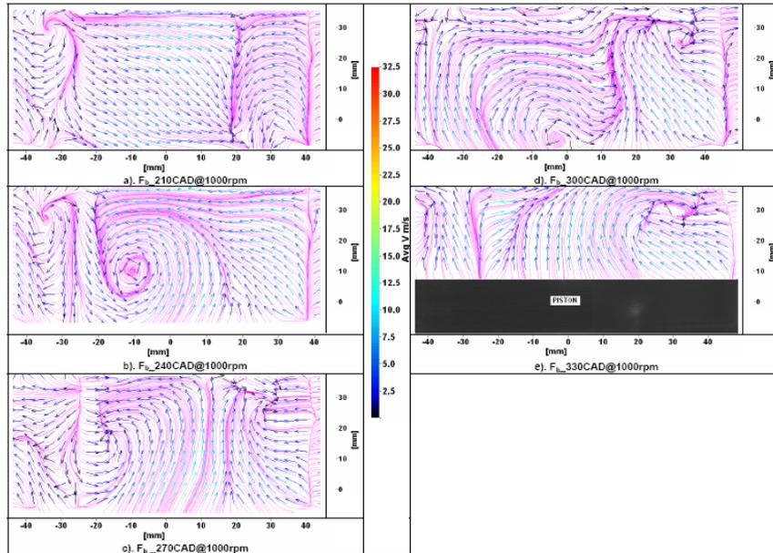
**Fig.6 The Ensemble Average Velocity Vectors of Flat-with-Bowl Piston During Compression**
