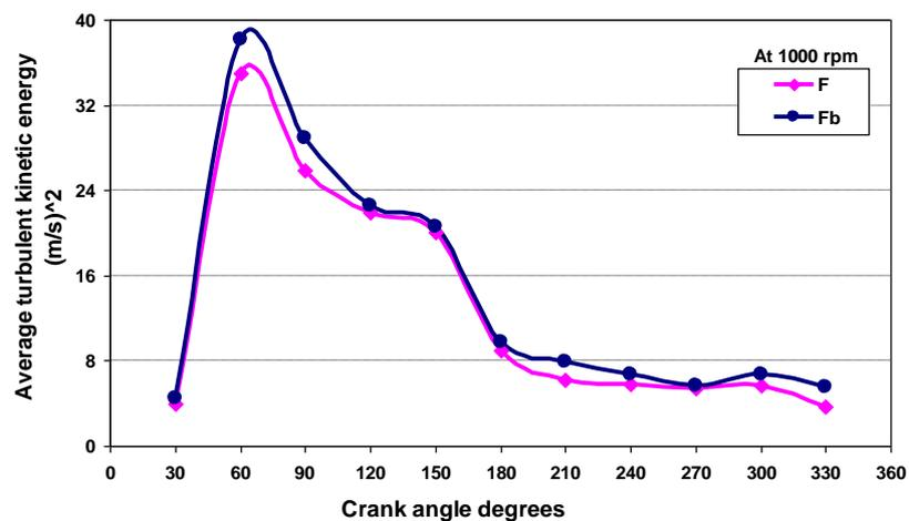
**Fig.8 Turbulent Kinetic Energy Against Various Crank Angles**
