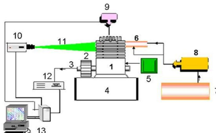
1. Engine, 2. Motor, 3. Encoder, 4. Test bench, 5. Speed controller, 6. Intake plenum,
