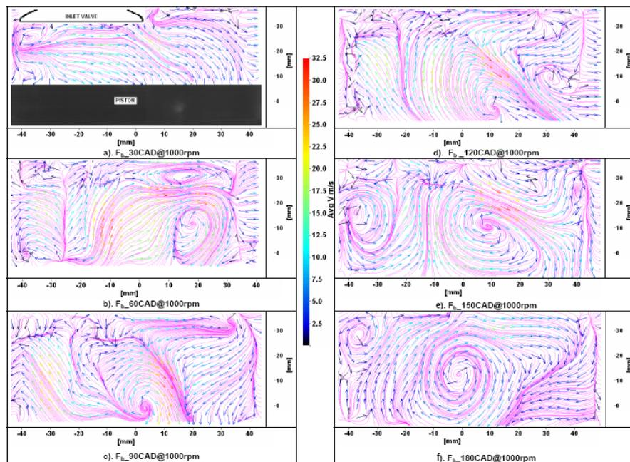
**Fig.4 The Ensemble Average Velocity Vectors of Flat-with-Bowl Piston During Intake Stroke**
