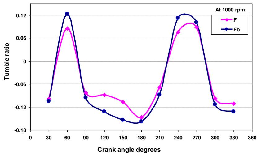
**Fig.7 Tumble ratio with Crank Angle Positions**
