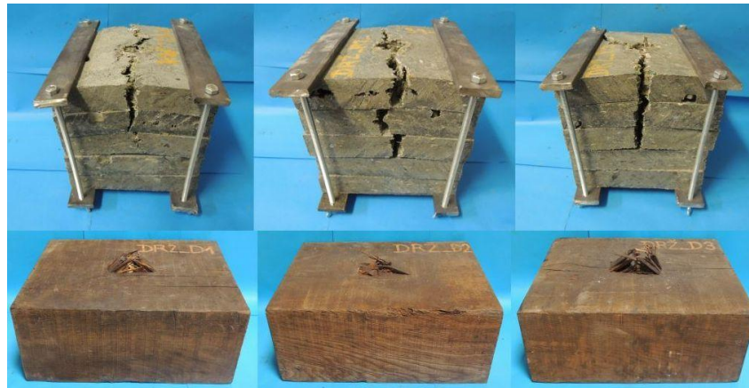
Figure 7: The specimens made of recycled plastic and of oak wood after conducting the screw spike pullout test
