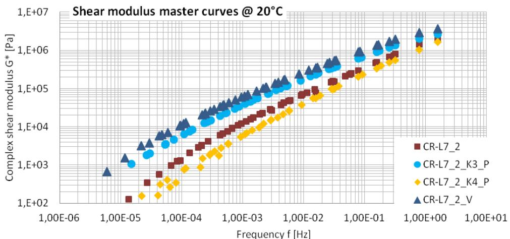
**Figure 7: Master curves for CRmB binders with different chemical additives; ref. temperature 20°C**
