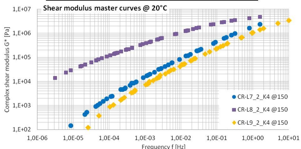
**Figure 5: Master curves for CRmB binders with selected pulverized rubber variants; ref. temperature 20°C**
