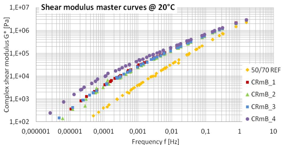
**Figure 4: Master curves for CRmB binders with pulverized rubber of 0.1-0.3 mm size; ref. temperature 20°C**
