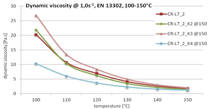
**Figure 2: Viscosity curves for CRmB binders with different catalysts; shear rate  $1.0 \text{ s}^{-1}$**
