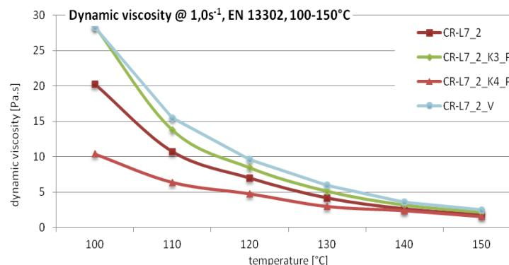
**Figure 3: Viscosity curves for CRmB binders with selected additives; shear rate  $1.0\text{ s}^{-1}$**
