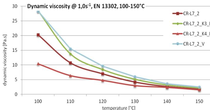
**Figure 3: Viscosity curves for CRmB binders with selected additives; shear rate 1.0 s<sup>-1</sup>**
