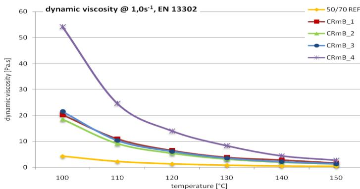
**Figure 1: Viscosity curves for CRmB with pulverized rubber of 0.1-0.3 mm size; shear rate  $1.0 \text{ s}^{-1}$**
