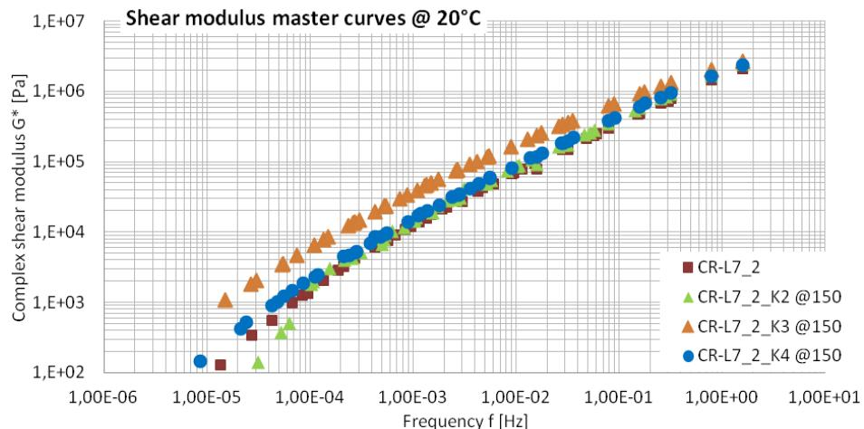
**Figure 6: Master Curves for CRmB Binders with Different Catalysts; Ref. Temperature 20°C**
