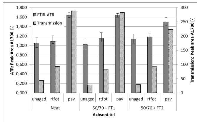
Figure 13: Peak areas of FTIR spectra in the carbonyl range (1720 – 1670 cm<sup>-1</sup>) at different aging stages
