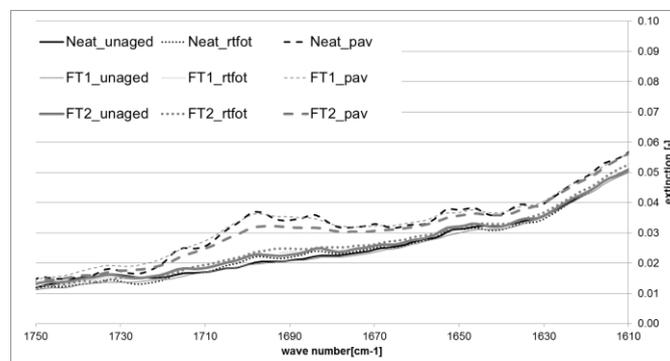
Figure 12: FTIR spectra (detail in  $1700\text{cm}^{-1}$  range) of unaged and aged binders in ATR technique
