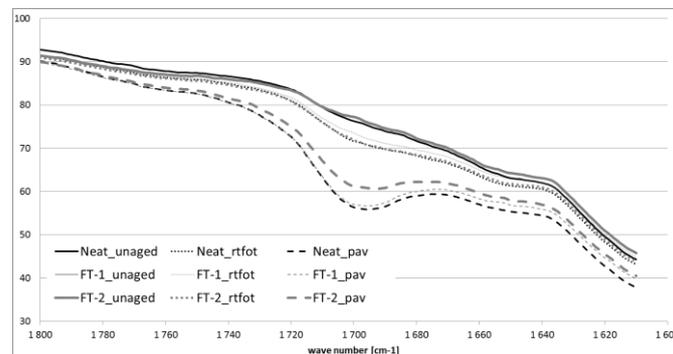
Figure 11: FTIR spectra (detail in  $1700\text{cm}^{-1}$  range) of unaged and aged binders in transmission technique
