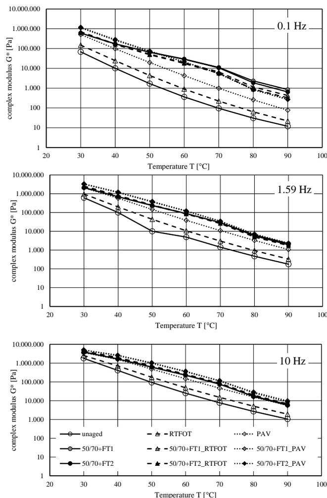
**Figure 3: Complex modulus versus temperature measured at 0.1 Hz (top), 1.59 Hz (middle) and 10 Hz (bottom)**
