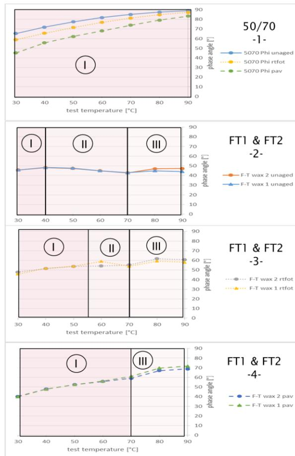
Figure 17: Effect of F-T wax based on phase angle
