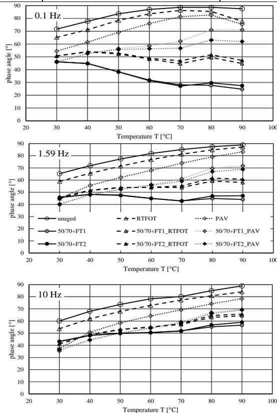
**Figure 4: Phase angle versus temperature measured at 0.1 Hz (top), 1.59 Hz (middle) and 10 Hz (bottom)**
