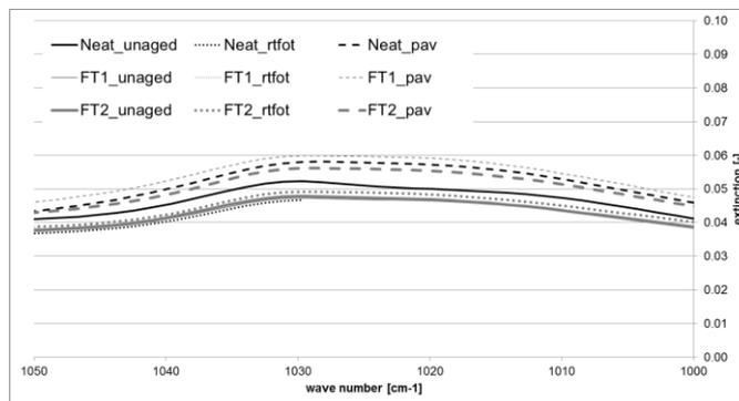
Figure 14: FTIR spectra (detail in 1030 cm<sup>-1</sup>) of unaged and aged binders in ATR technique
