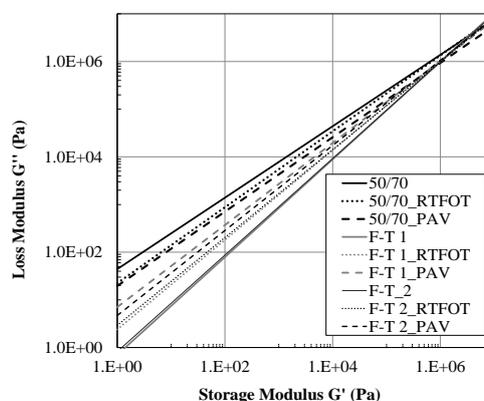
Figure 6: Regressing curves of the straight and wax modified bitumen samples at varied aging stages in the Cole-Cole-plot
