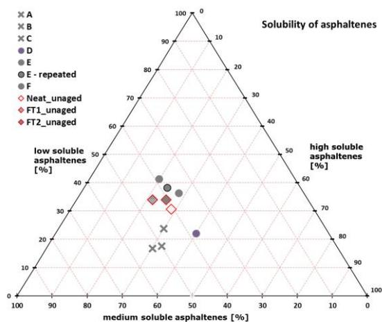
**Figure 16: Comparison between asphaltene components by [10] of different 50/70 bitumen types**
