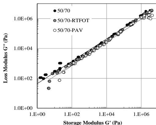
Figure 5: Cole-Cole-plot of the DSR-temperature-frequency sweep tests obtained on the unaged, short- and long-term aged samples of the straight bitumen 50/70 – addition of fitting curves
