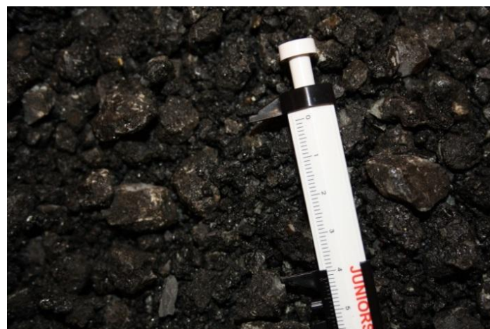
Figure 2: Multiple aged and crushed RAP.
