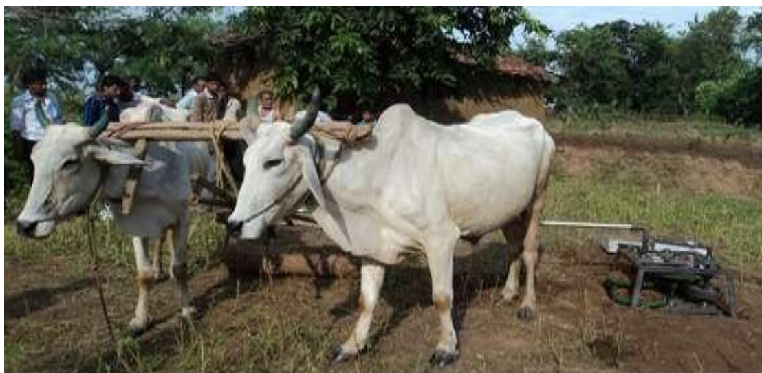
Fig.3 Animal powered mechanical device for home lighting system.
