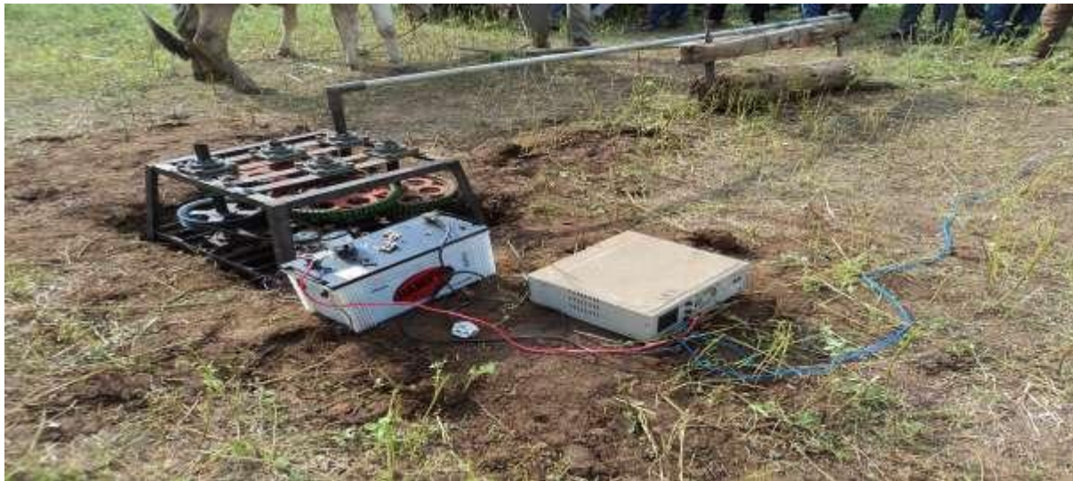
Fig1: Integrated Belan, Mechanical link, Speed Icreaser, belt & pulley, alternator and battery
