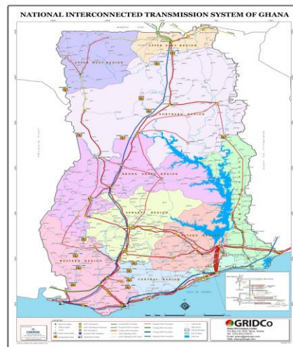
Figure 2: National transmission system of Ghana [http://www.gridcogh.com/en/national-grid.php].
