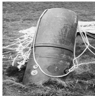
Fig.4. German parachute-retarded magnetic mine.
