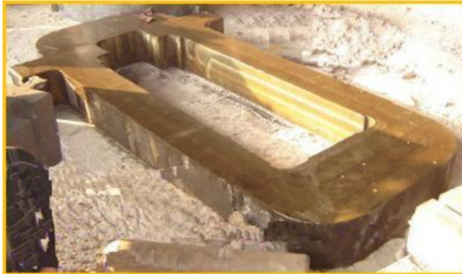
Fig. 2.1: Housing of rolling mill
