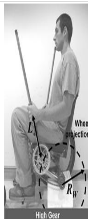
Fig 2. LFC variable mechanical advantage drive train
