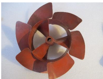
Fig 2.3.3 Turbine of turbo generator
