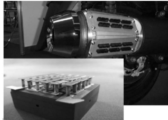
Fig 2.2.3 TEG modules mounting to the exhaust
