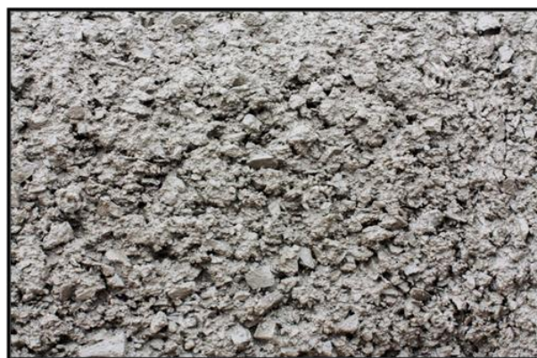
Fig.1 Concrete in plastic state
