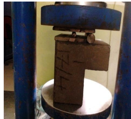
FIG 4 Shear test specimen
