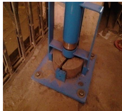
FIG 6 Impact test machine with Impact specimen
