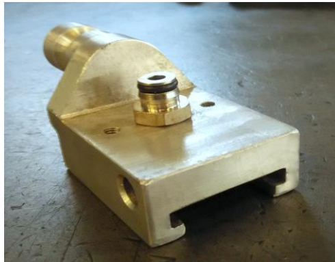
Fig.6.3.2 Manufactured suction pad attacher with mounting elements.
