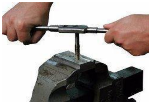
Fig. 2.2.1 Conventional Tapping Process
